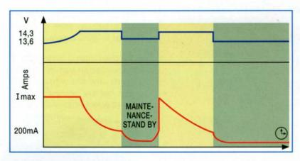
long-term maintenance of batteries while out of service.
